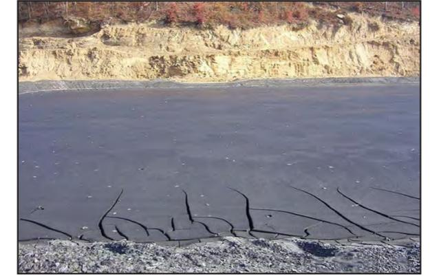
**Figure 4** – Adjacent treated Slurry cell after three (3) weeks.
