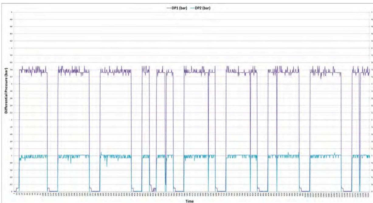
**Figure 4** – Graph showing Differential Pressure (DP) across two stages of the RO system.
