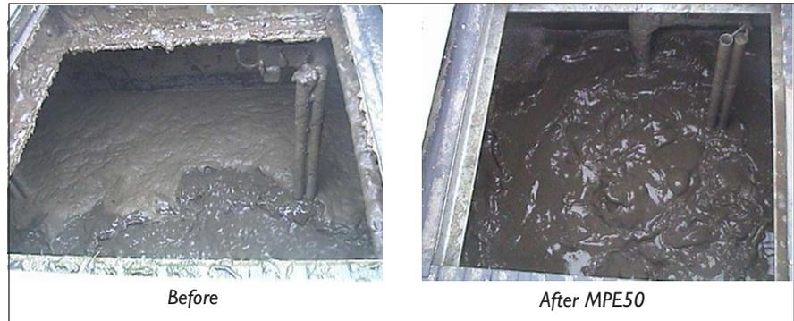
Figure 3 – Comparison of the foam levels before and after MPE50 addition (no tidal ingress at the time of the photographs).
