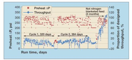
Figure 4 Rapid fouling because the storage tank was not nitrogen blanketed
