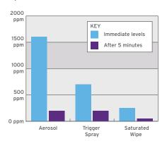
\*TECHNICAL REPORT - TR9902R Investigation into Airborne Concentrations of Alcohol when using a Trigger Spray, and Aerosol and Saturated Wipes
