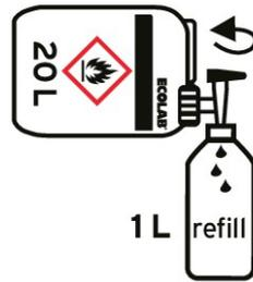
6. Consider using a drip tray around packaging and bottles. Open tap and fill refill bottle. Always decant into the Ecolab labelled bottles supplied and has to be labeled with the product name, shelf life information and date of refilling.
