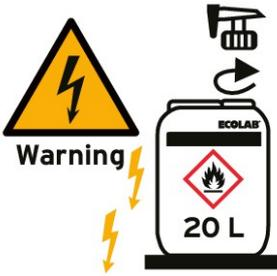
5. Attention: Carefully read the safety instructions below. Secure grounding before handling/ opening canisters. Open 20 L canister for the refill procedure only and screw on filling tap. Place the canister on its side at an elevated position with the valve in the lowest position.
