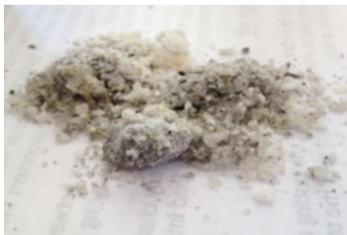
Figure 1 - Sample of a steam system deposit that was analyzed to be cyclohexylamine carbonate.
