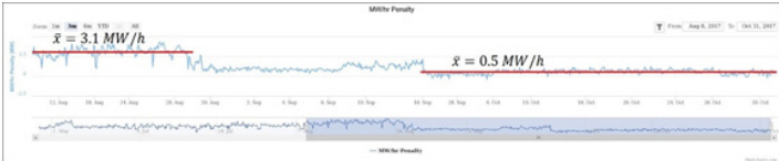
Figure 5: MW Penalty declined 2.6 MW/hr after the air leaks were repaired.
