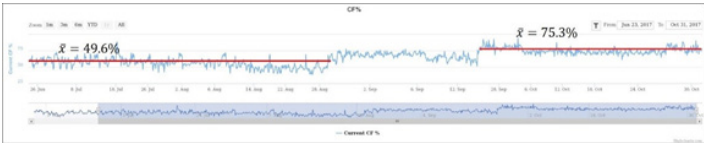
Figure 6: Cleanliness Factor increased 25.7% following the air leak repairs.
