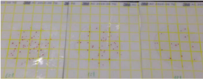
BL3 1 temperature zone after Nalco Water treatment BL3 2 temperature zone after Nalco Water treatment BL3 3 temperature zone after Nalco Water treatment
