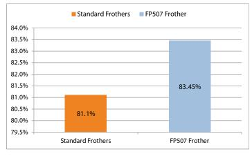
Figure 1. FrothPro $^{\text{TM}}$  507 Increased Copper Recovery by 2.4% versus Standard Reagent in the plant
